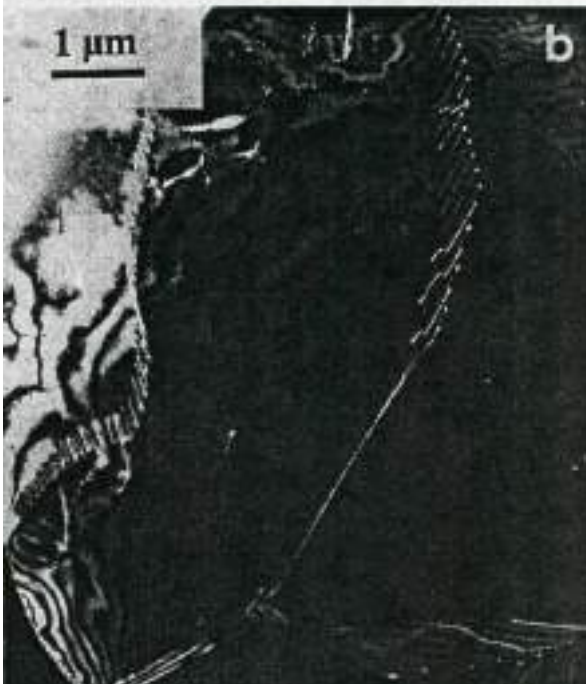
Figure 7.25. A bright field image of a large number of parallel dislocation lines in olivine. The dislocation lines are inclined to the surface of the thin specimen and hence appear as short segments, the ends of the dislocation lines marking their intersection with the top and bottom of the specimen.
