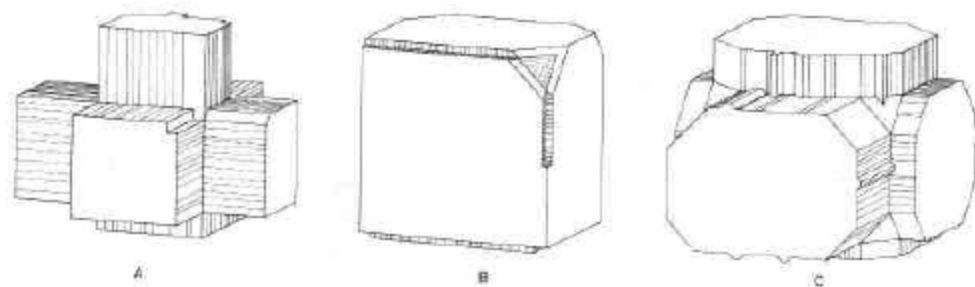
FIG. 3. Idealized drawings to emphasize certain variants of habit of pyrite crystals from the Westvaco mine, Wyoming. Each is based on observations on particular crystals and all are drawn to the same scale. The drawing at right represents a crystal with total width of about 0.4 mm. The striations in all cases are schematic only.
