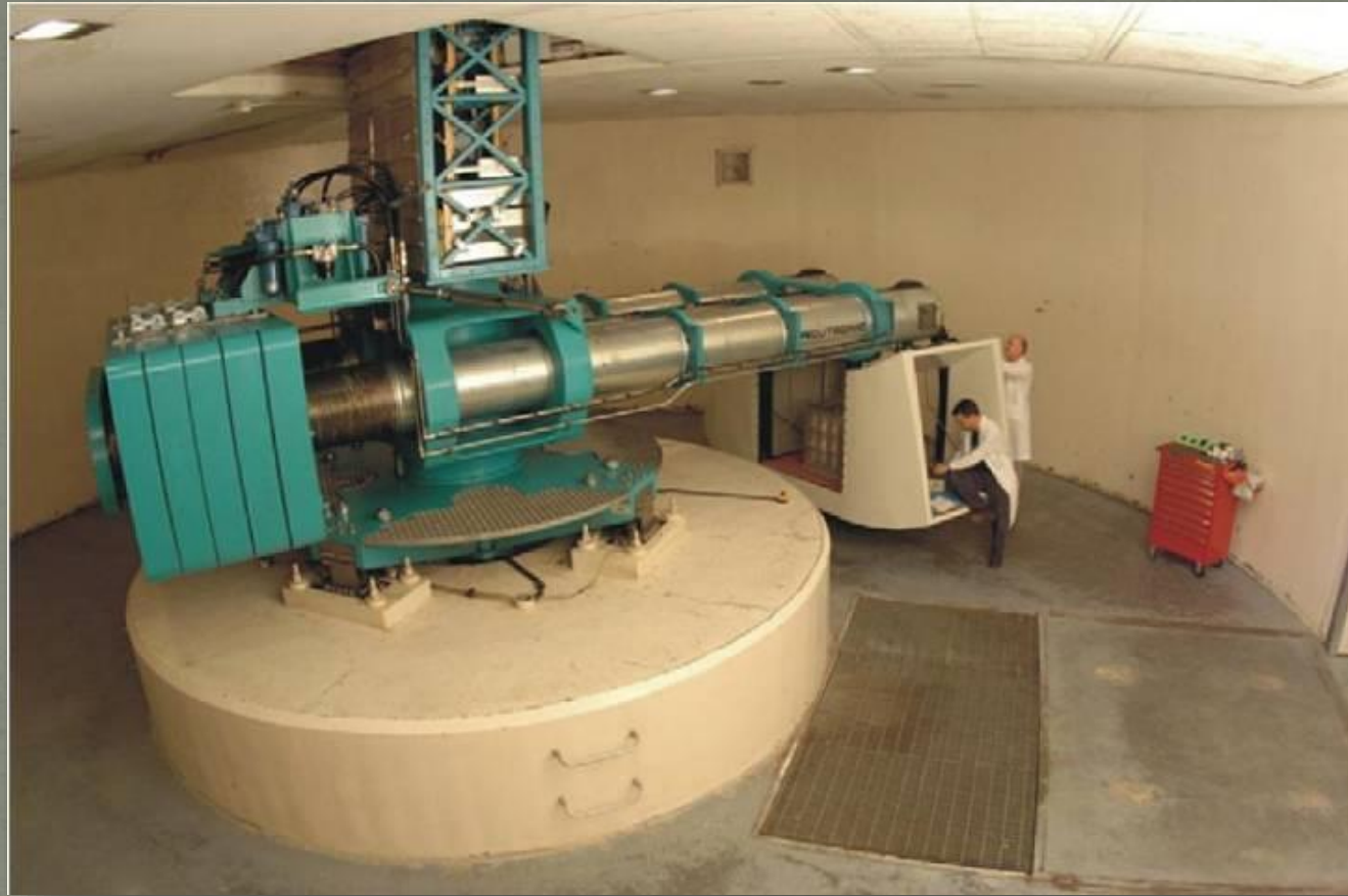
The C-CORE Accutron 680-2 centrifuge Experimental Tectonics Laboratory, Department of Geological Sciences, Queen's University, Kingston, Ontario, Canada ( Noble, Dixon, 2011 )
